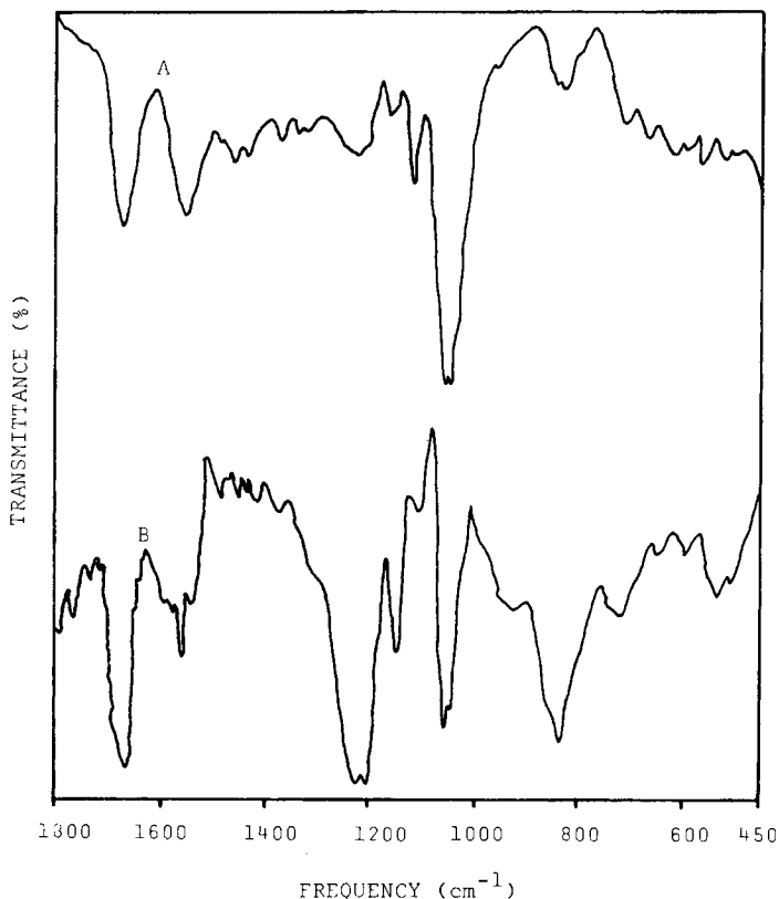
Fig. 6. Interferometer spectra of Pyrovatex finish on cotton fabric after Weather-Ometer exposure to \text{SO}_2 : A, 165 hr, xenon arc light, washed; B, 150 hr, no light, washed.
